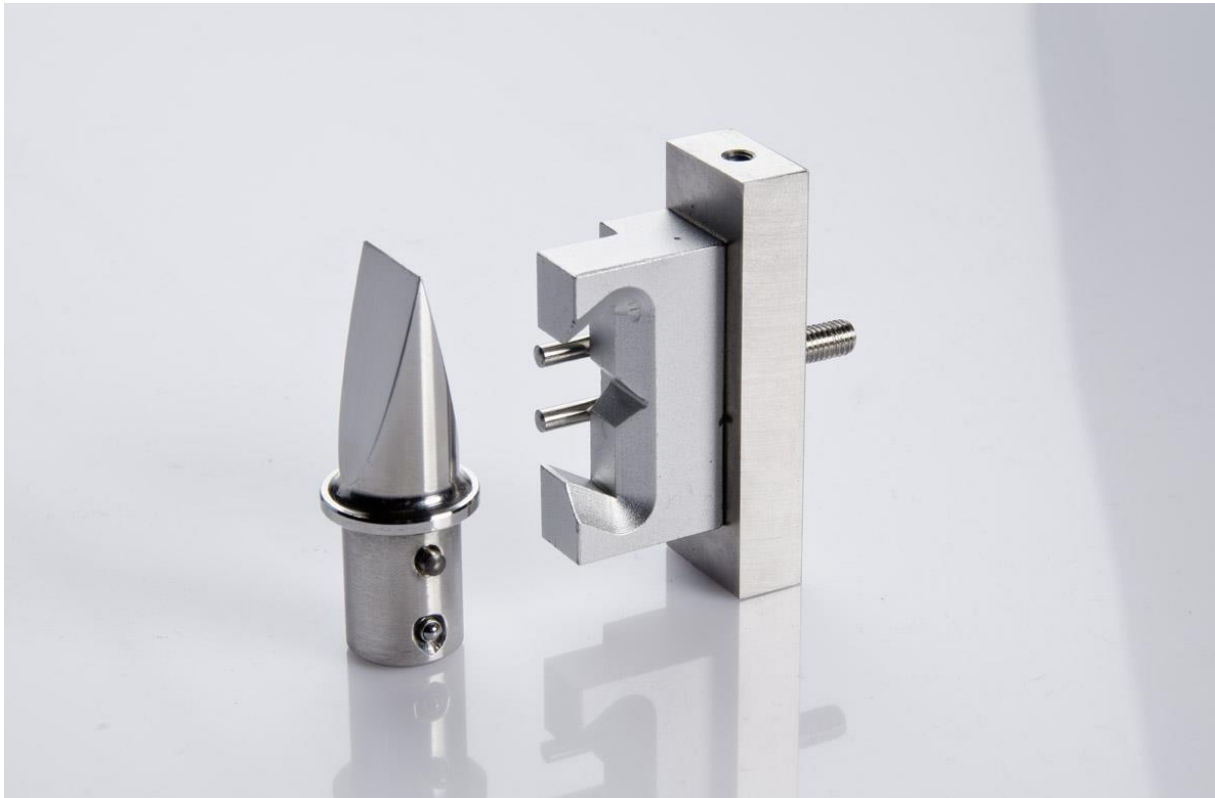
Tension Strength Test Set to test tablets having a break-line
